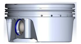
There are 2 locks per piston. Take one wire lock and locate the end in the relief notch in the piston pin hole at 90 degrees from the pick lock groove.
