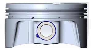
Using a piston pin, simply slide the pin into the piston and push it against the lock, making sure the lock does not move. It is a good idea to press the pin against both sides of the wire lock to check engagement
