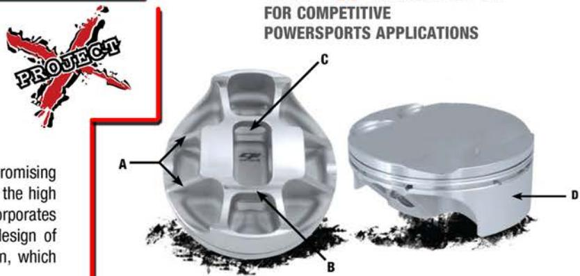
**A**- External bracing minimizes piston deformation to maintain maximum ring support to deliver more power.
