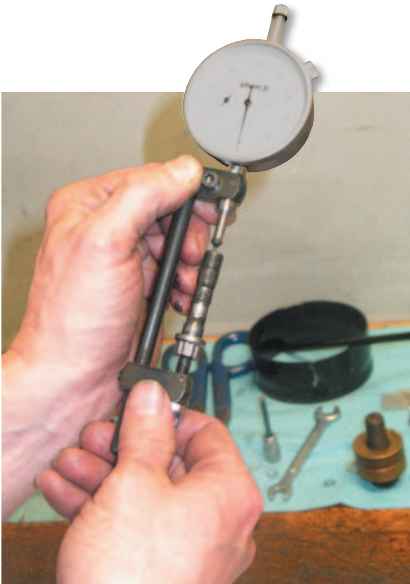
Ken Troutman of KT Engine Development demonstrated the process of checking rod bolt stretch for us. Step number one is to put the bolt in the gauge and zero out the dial.
