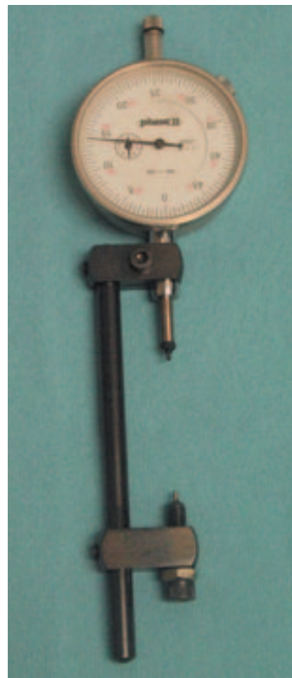
Although it can be done with different styles of calipers, a dedicated bolt stretch gauge is designed to do its job while the rod is installed in the engine. It will make your life easier.
