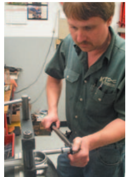
Next, he secures the rod in a rod vise, makes sure the bolt is properly coated in lubricant, and torques it to a number just under his target figure.
