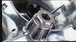
Integrated idle bypass valve for full idle control
