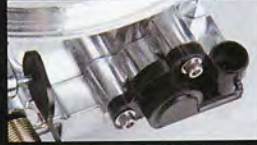
Factory ready TPS mounting points for use with data acquisition
