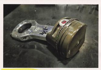
Bryan Moreland of CP-Carrillo remarks that in designing its pistons as used by JFR it has concentrated on stabilisation within the bore, and he notes that around BDC is the most problematic owing to the stroke. The key to this stabilisation is in the geometry of the piston above the skirt area; he declines to be more specific than that
